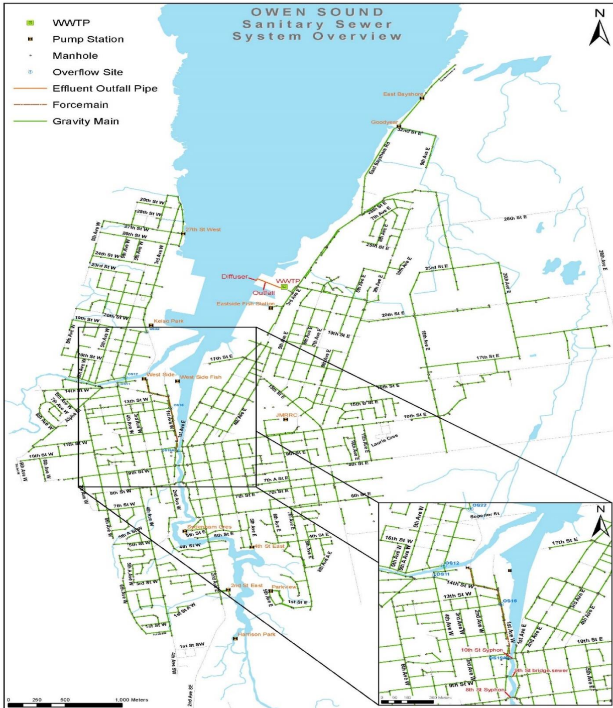
Figure 23: Overview of the City's wastewater network
