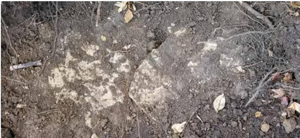
Photo 4: View of bedrock surface in TH-5. Note soil-infilled epi-karst fracture.
