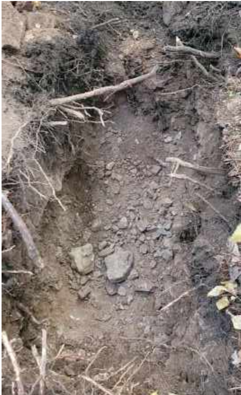
Photo 6: View of bedrock surface in TH-1.
