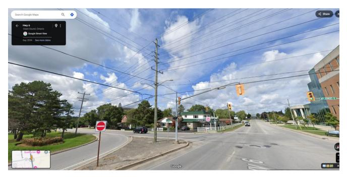
Google Street View looking northwest, the hydro pole in the centre of the image is considered a fixed object in any reconstruction design. Note the number of lines attached in each direction; approximately 40 total.
